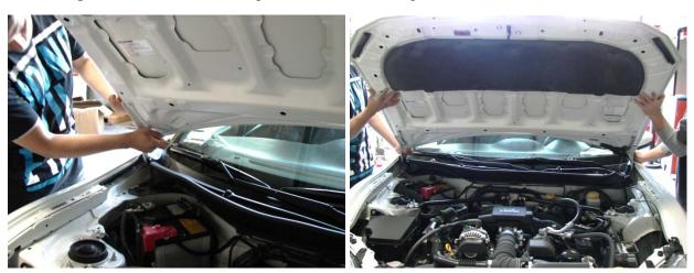
**Step 3:** Proceed to the Seibon Carbon hood. Carefully flip the hood over so that you are able to see the underside of the hood. Use a wrench to remove the wooden legs. In some cases, you may need to transfer your OEM striker onto your new carbon fiber hood. To do this, simply unbolt the striker and screw it onto the carbon hood.
