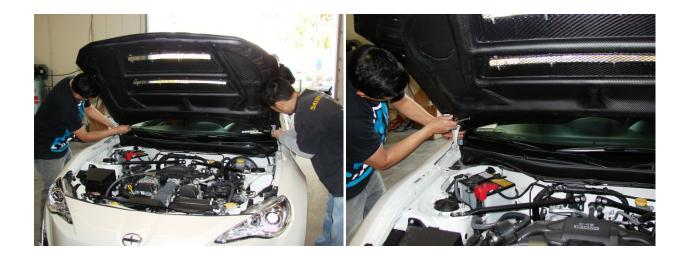
**Step 5:** Before closing the hood, make sure that there are no tools left in the engine bay and then proceed to slowly lower the hood while you and a partner watch for fender clearance. Close the hood carefully-slamming the hood may cause damages. Check alignment of the hood and latch.
