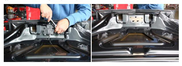
**Step 8:** If applicable, install license plate lights and tail garnish onto the Seibon Carbon trunk. (Note: light holes are intentionally made smaller than OEM trunk to ensure a snug fit. To resize, use a file.) Otherwise, proceed to install your OEM latch onto the carbon trunk using your OEM screws, clips, etc. In some cases it may be necessary to enlarge holes to ensure a snug fit.
