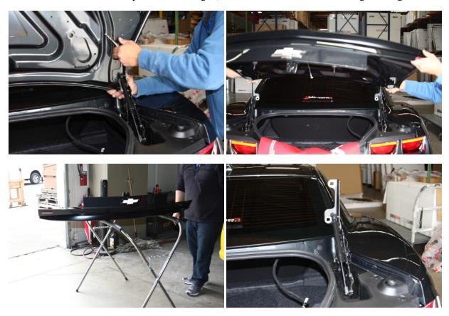
**Step 5:** You should perform a quick test fit of the carbon fiber trunk. The Seibon trunk should already be open and inspected for shipping damage upon delivery from the trucking company. Remove the wooden legs from the trunk. Place the trunk where it will be easy to work with.
