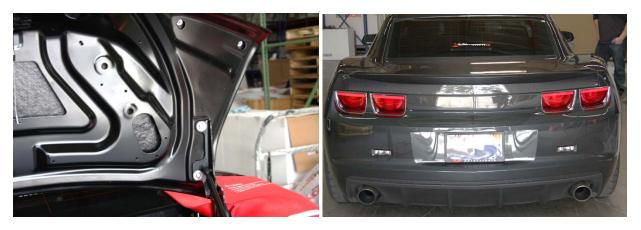
**Step 7:** Go back to the OEM trunk. Carefully proceed to remove the trunk's latch and bump stops. If applicable, remove license plate lights and garnish.
