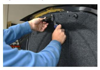
**Step 3:** Remove the trunk cover. After removing the trunk cover you should be able to see the taillight harness. Proceed to carefully detach the taillight harness/tail lights from the *trunk*. The tail light harness should be left attached to the *car*.
