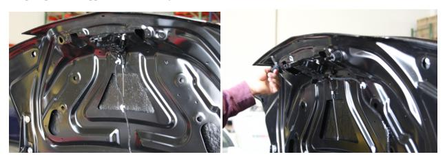
**Step 11:** Reinstall the trunk cover, if applicable, and finish the emergency trunk release hook and latch if these weren't completely finished.
